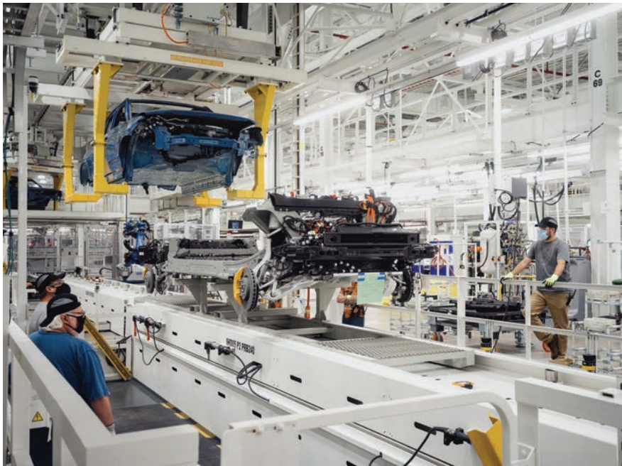
Rivian's R1T tophat and skateboard are married at the start of the trim build at the company's plant in Normal, Illinois.
